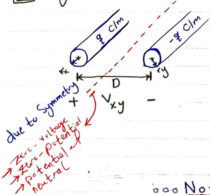
$$\begin{aligned} V_{xy} &= \frac{1}{2\pi\epsilon} \left[ q \ln \frac{D_{xy}}{D_{xx}} - q \ln \frac{D_{yy}}{D_{xy}} \right] \\ &= \frac{q}{2\pi\epsilon} \ln \frac{D_{xy} D_{xy}}{D_{xx} D_{yy}} \\ &= \frac{q}{\pi\epsilon} \ln \frac{D}{\sqrt{r_x r_y}} \text{ Volts} \end{aligned}$$
