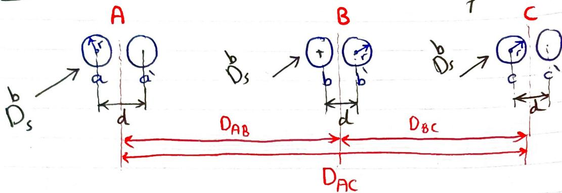
$$D_{AB} = \text{GMD}_{A,B}, \quad D_{BC} = \text{GMD}_{B,C}, \quad D_{AC} = \text{GMD}_{A,C}$$
